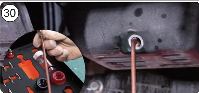
30. Connect hook adapter into the oil pan's drain hole, connect the black hose to the hook adapter and turn on its valve, then turn on the vacuum regulator to finish suctioning the oil that remains in the oil pan that could not been drained out naturally (this depends on the oil pan construction).
