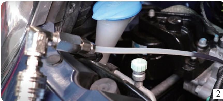
6. Extract all the used oil from the vehicle. Once extracted close the black hose valve and turn off the regulator.
