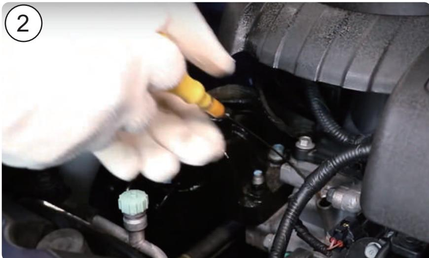
2. Remove the engine oil dipstick.
