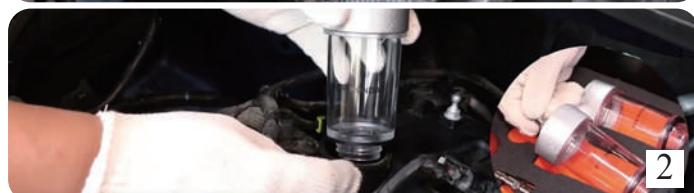
11. Remove the vehicle's engine oil filling cap and chose the most suitable engine oil filler neck transparent chamber or the universal adapter, then install it onto the engine, and connect the 90-degree adapter if necessary.
