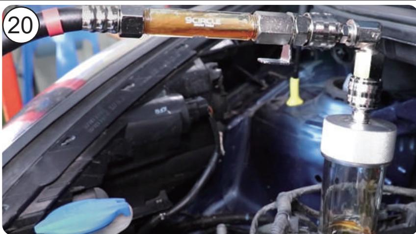
20. Pour out the remaining oil in the hose and machine into the engine. Then turn off the flush chamber pressure regulator.
