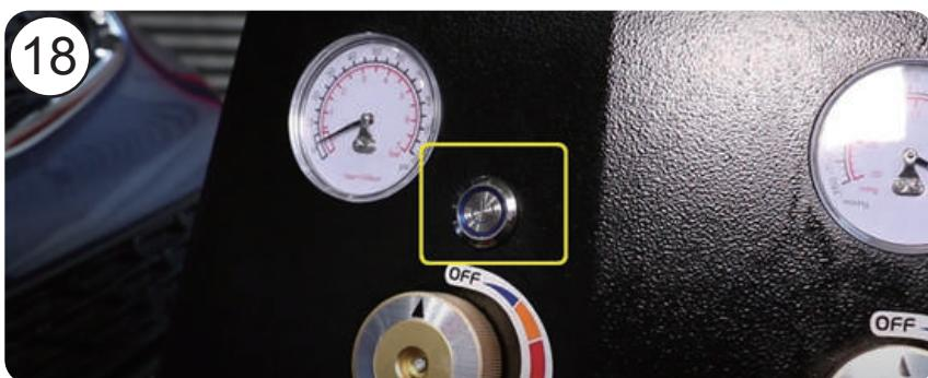
18. Switch off the motor of the flush chamber.
