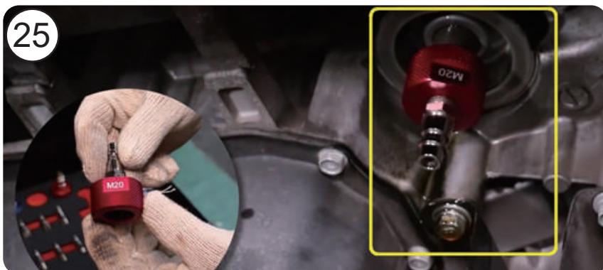
25. Connect the most suitable oil filter adapter.
