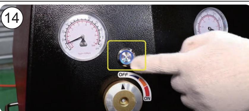
14. Turn on the motor of the flush chamber.
