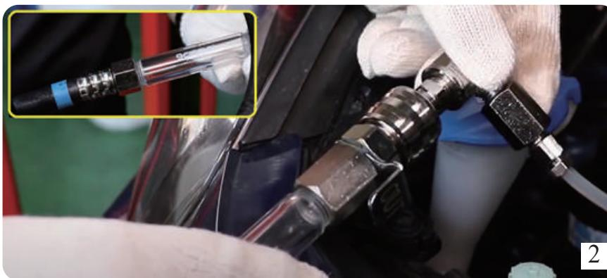
9. Fill flush oil into the 2L tank and turn on the motor of the 2L tank.
