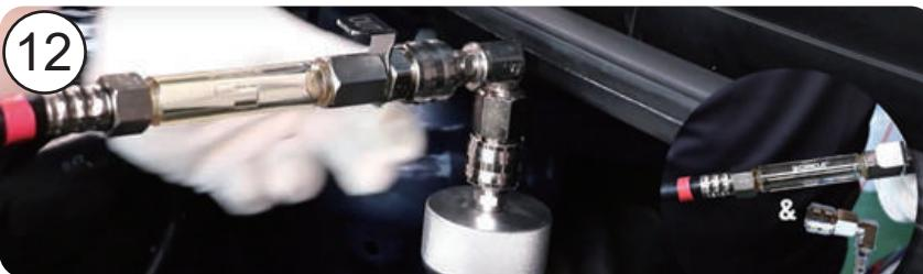
12. Connect the red hose into the chamber adapter and turn on its valve.
