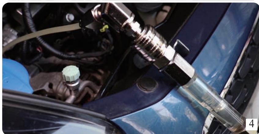
10. Once all the flush oil is sent into the vehicle, turn off the blue hose valve, and disconnect it from the Teflon tube.
