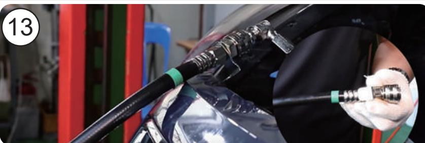
13. Connect the green hose into the Teflon tube and turn on its valve.
