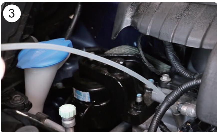
3. Install the Teflon tube as the same length as the dipstick.
