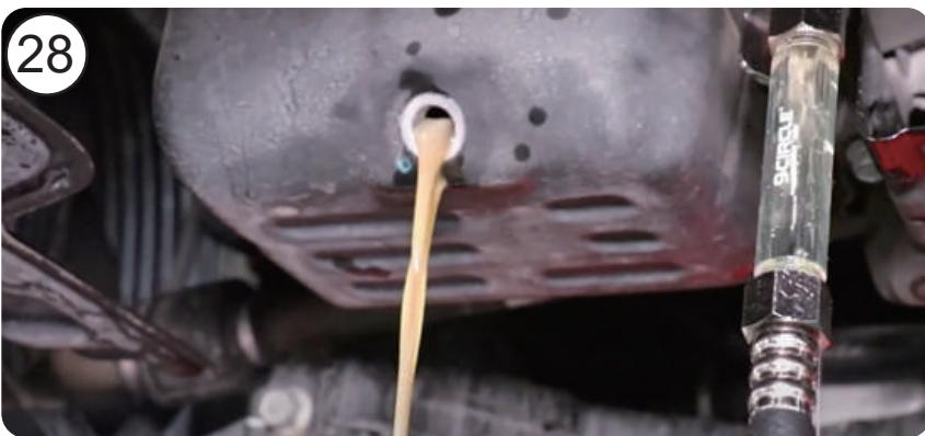
28. Remaining oil in the 2L tank will help to clean out the rest of the dirty oil from the vehicle.
