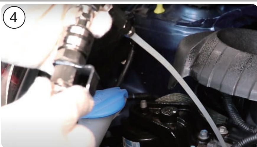
4. Connect the machine's 12L tank suction hose (black hose, the one without color mark) to the Teflon tube and turn on its valve.
