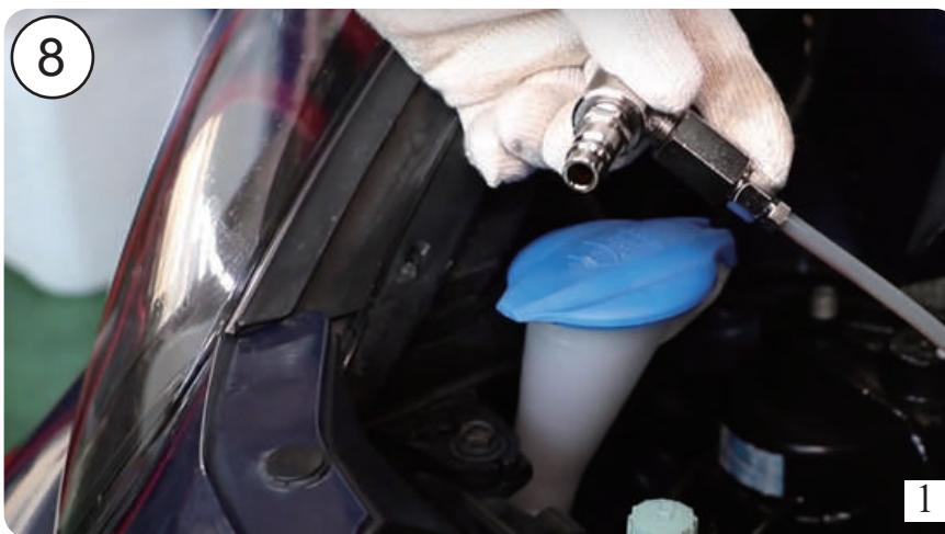
8. Disconnect the black hose from the Teflon tube and install the 2L tank pressure hose (blue hose) and turn on its valve.
