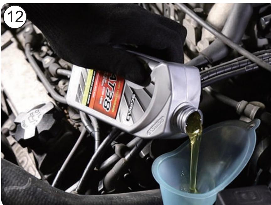
12. Once filling the ATF, remove the funnel and install back the dipstick.
