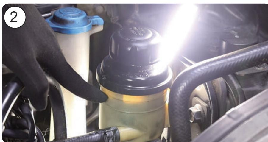
2. Check the level of the PSF with a LED light (for better accuracy) then open the PSF reservoir cap.
