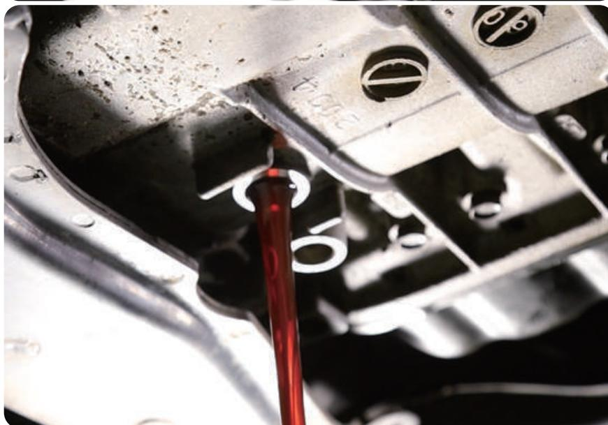
2. Remove the ATF pan drain plug and drain the ATF.
