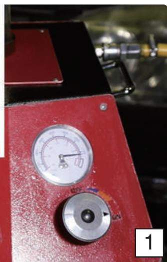
16. Turn on the machine's black valve, then add PSF to recommended level, then open black hose valve.
