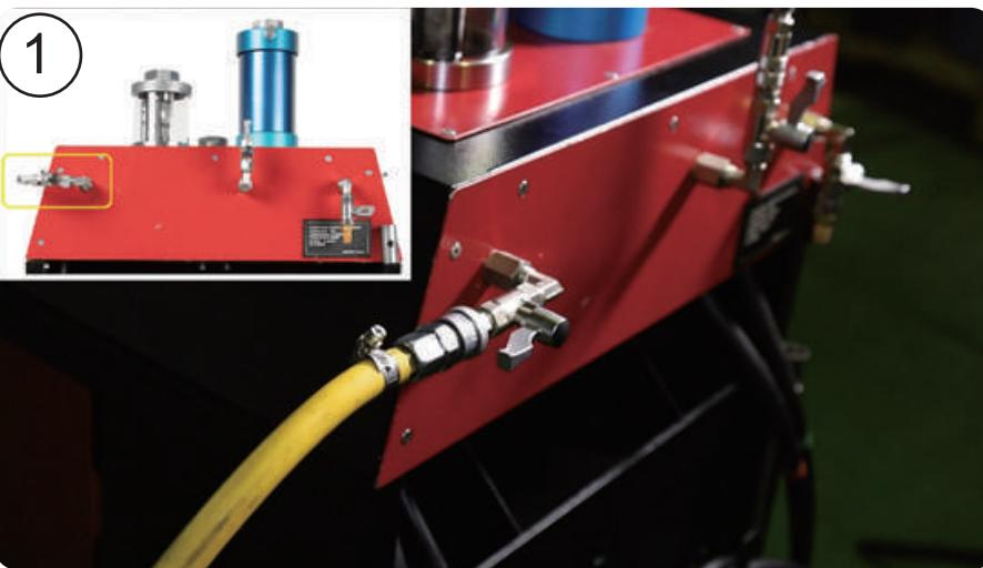
1. Connect air supply to the machine and turn on its valve.
