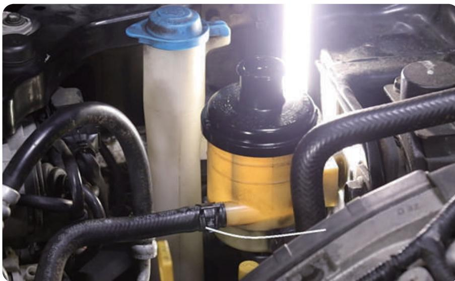
13. Remove the PSF reservoir return hose. On the PSF reservoir install an adapter hose with a stopper adapter, and on the PSF return hose install a step adapter.
