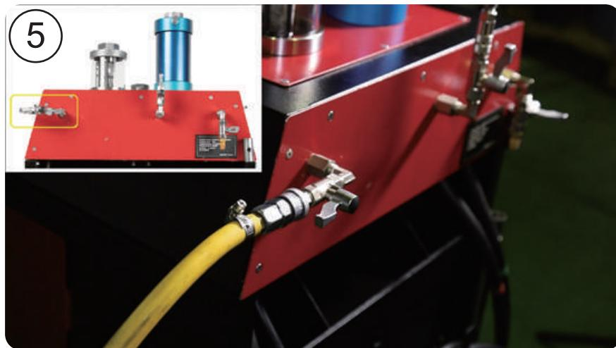
5. Connect the air supply to the machine and turn on its valve.
