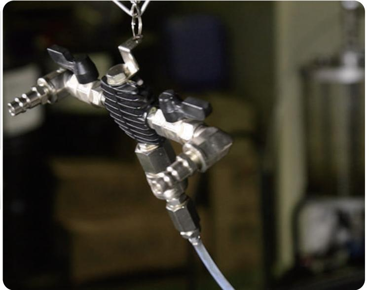
4. Connect the extension hose with transparent chamber to the black hose and connect it to whichever side of the T adapter and turn on the black hose valve and the T adapter valve.
