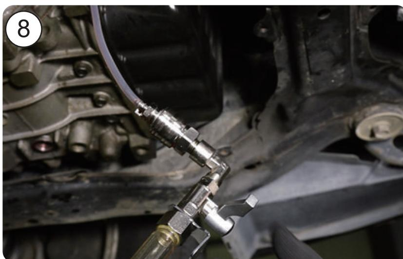
8. After all the ATF is drained, turn off the valve of the red hose and the machine's silver valve.
