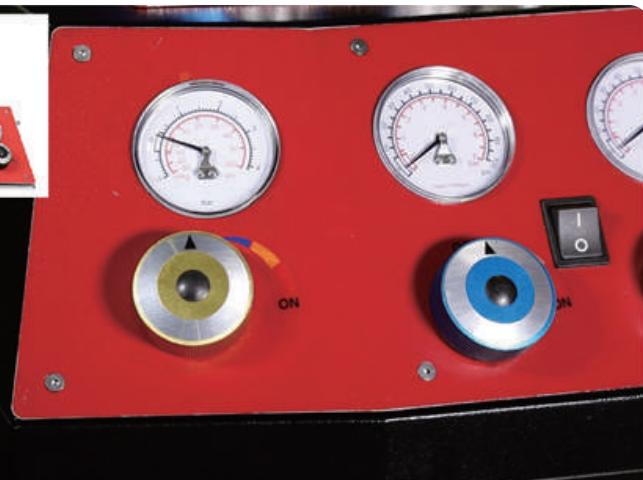
15. Once the ATF is sent from the machine to the vehicle turn off the golden valve then red hose valve and the T adapter valve.
