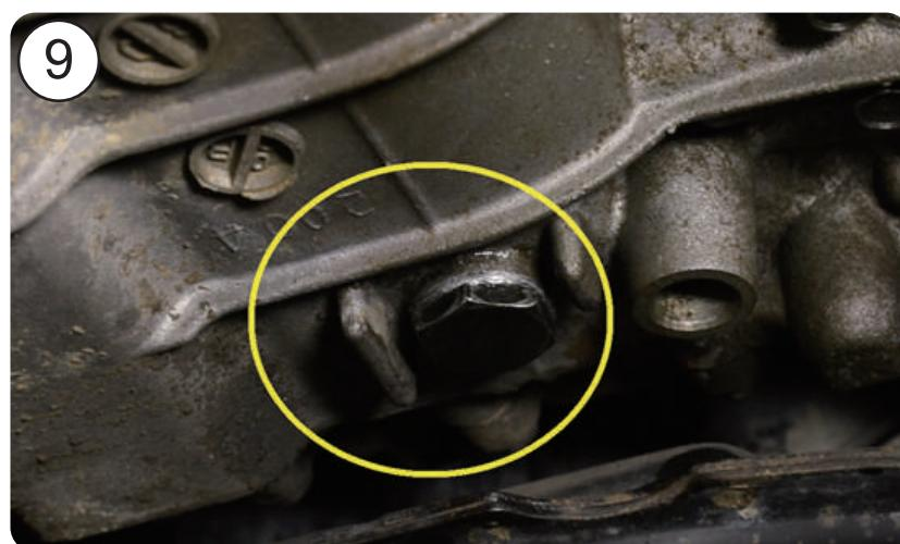
9. Install back the drain plug.
