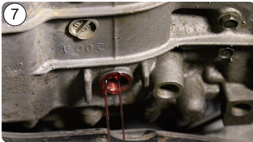
7. Air pressure will help to drain out all the remaining ATF that is hidden in difficult to access spaces which don't allow to drain the ATF in a standard procedure way.
