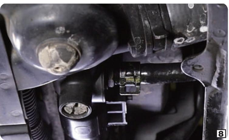
21. Remove the ATF pan drain plug and drain the remaining ATF of the vehicle.
