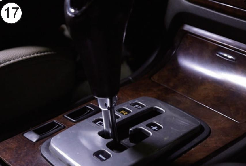
17. Turn on the vehicle for 2-3 minutes and use all shifts, then turn it off, this is to allow the ATF from the converter to pass through.
