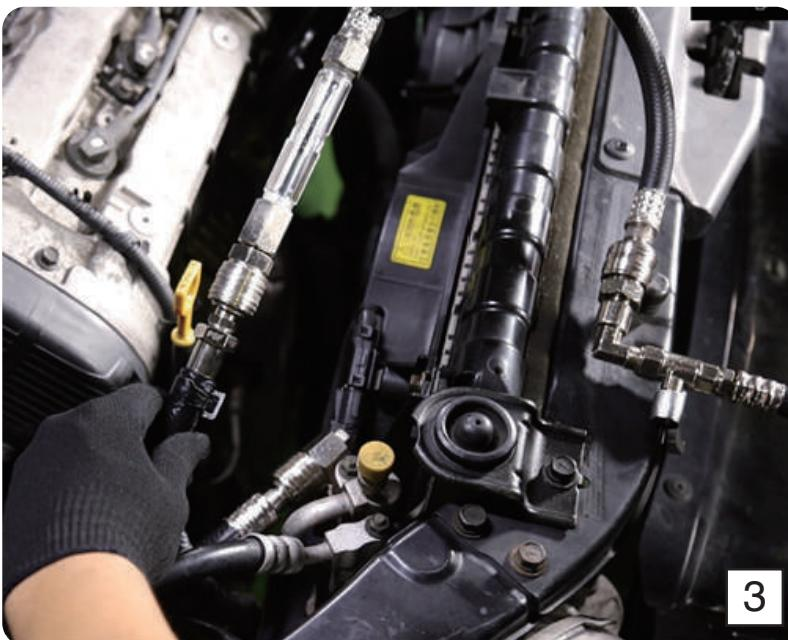
14. Install a hose with transparent chamber to the black hose and then into the step adapter (which is connected to the PSF Return hose).
