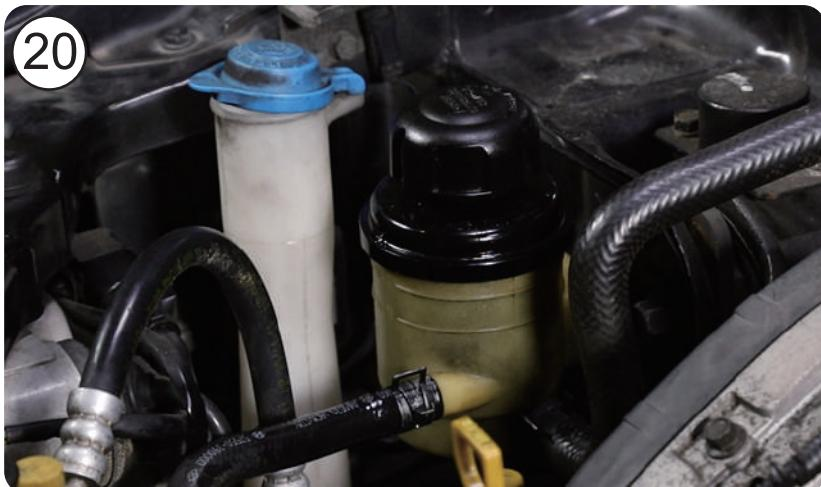
20. Once finish refilling the PSF, remove the funnel and install back the reservoir cap.
