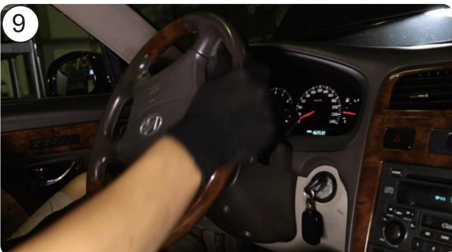
9. Turn on the vehicle and turn the steering wheel for couple of minutes to clean the steering system. Then turn off the vehicle.
