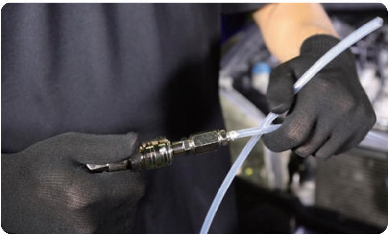
10. Connect a Teflon tube to the black hose. And turn on the machine's black valve.
