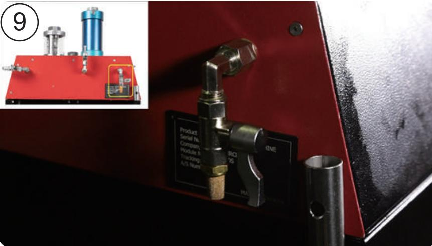
9. Turn on the machine's rear right valve, then turn on the front golden valve.
