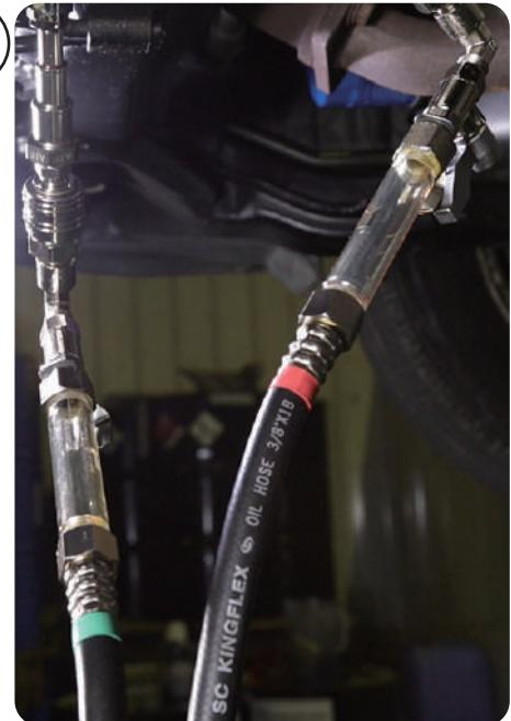
13. Have to find out which of the two adapters will be OUT (ATF goes from the vehicle to machine) and which one will be IN (ATF goes from machine to vehicle), so connect the red hose and green hose to the adapters, and turn on its valves. At this point, does not matter which hose is connected to which adapter.
