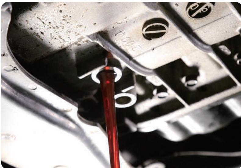
24. Once is done, lift down the vehicle, remove the ATF dipstick, put a funnel, and fill out 350ml of AT38 (A/T Stop Slip / Stop Leak Protection) and the recommended ATF at the suggested level by the vehicles manufacturer.
