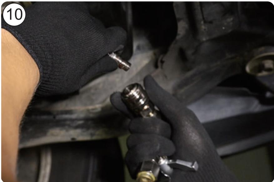
10. Disconnect the red hose from the adapter and remove the adapter and install back the bolt.
