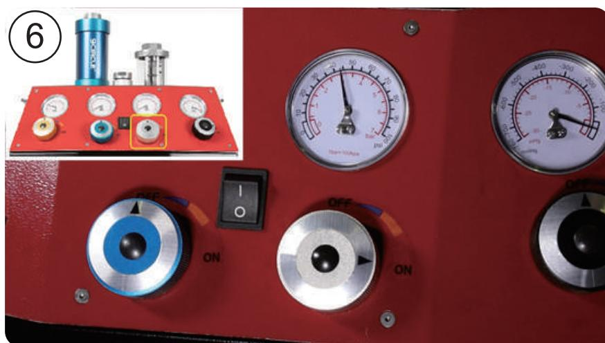
6. Turn on the machine's silver valve and the red hose valve to drain out the rest of the ATF.
