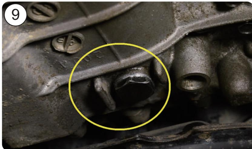
7. Air pressure will help to drain out all the remaining ATF that is hidden in difficult to access spaces which don't allow to drain the ATF in a standard procedure way.
