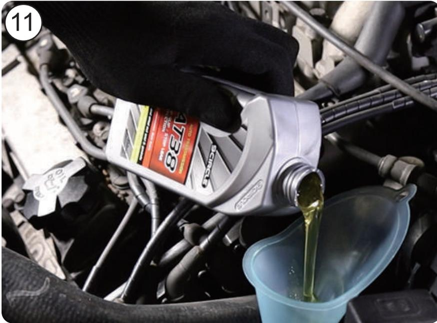
11. Once is done, lift down the vehicle, remove the ATF dipstick, put a funnel, and fill out 350ml of AT38 (A/T Stop Slip / Stop Leak Protection) and the recommended ATF at the suggested level by the vehicles manufacturer.
