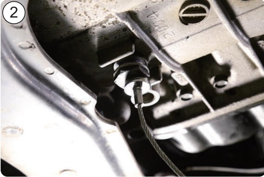
2. Remove the ATF pan drain plug and drain the ATF.
