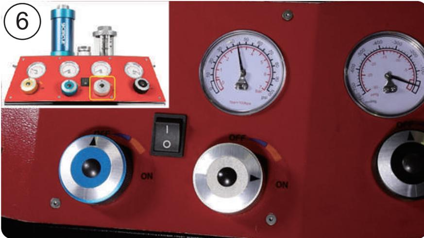
6. Turn on the machine's silver valve and the red hose valve to drain out the rest of the ATF.
