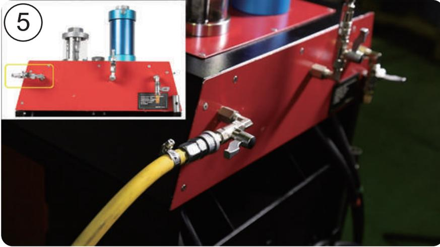
5. Connect the air supply to the machine and turn on its valve.
