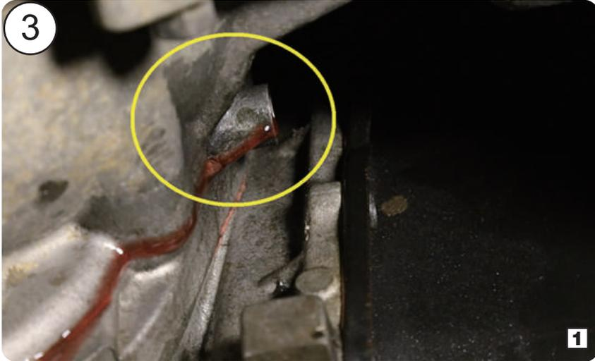
3. Remove the bolt and install the 90° adapter M8.
