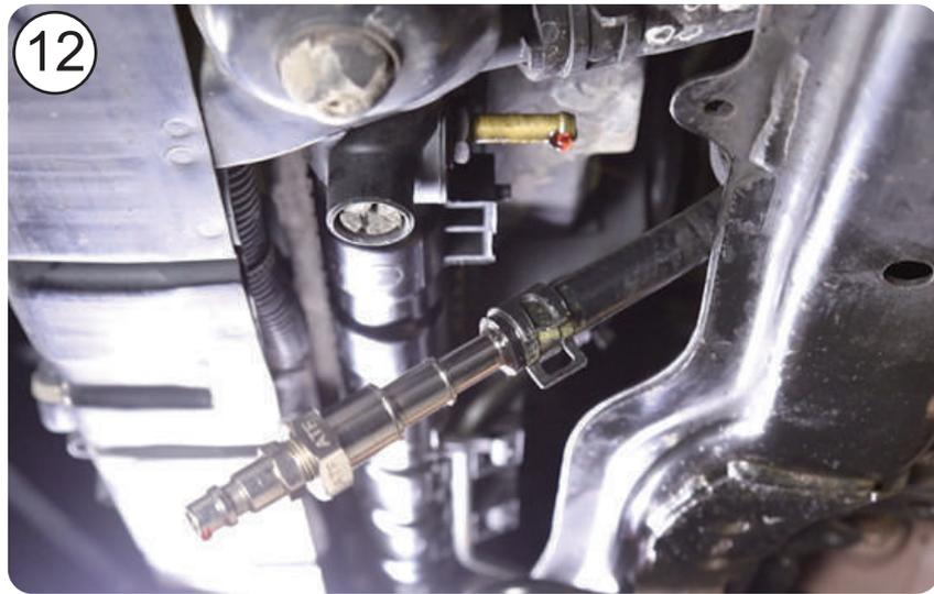
12. To the ATF's hose connect the ATF step adapter; and on the ATF's pipe, connect a hose adapter with its clamp.
