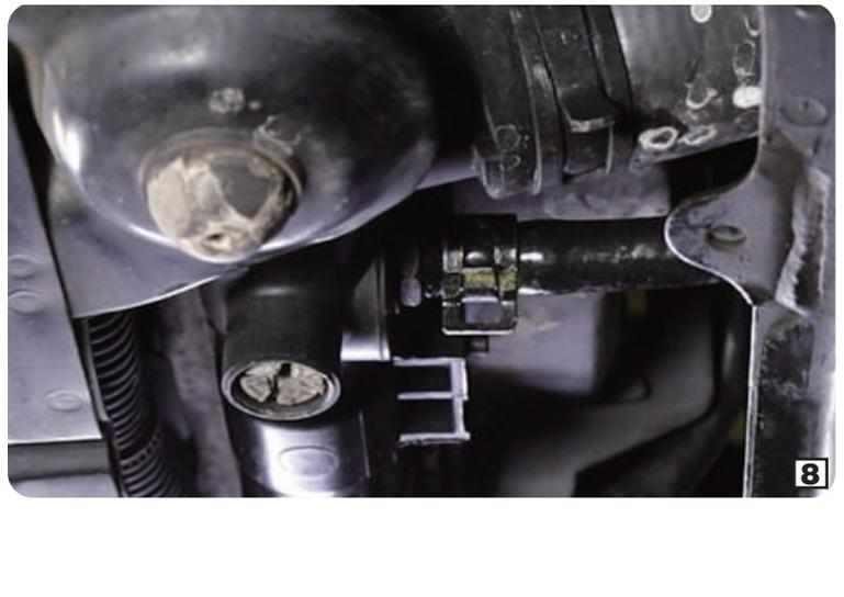
21. Remove the ATF pan drain plug and drain the remaining ATF of the vehicle.
