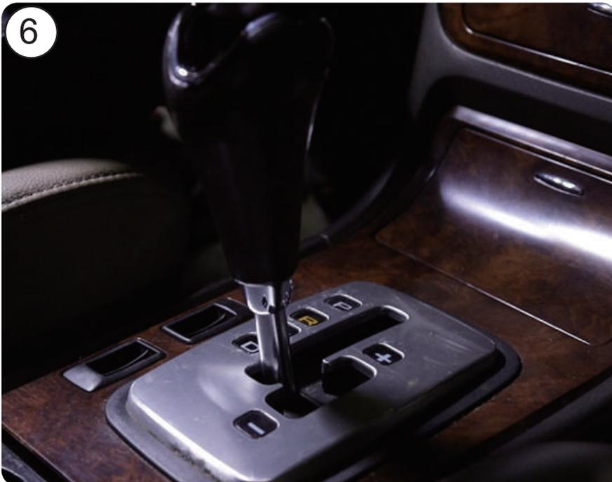
6. Turn on the vehicle and constantly use all shifts on the transmission for about 2 minutes.
