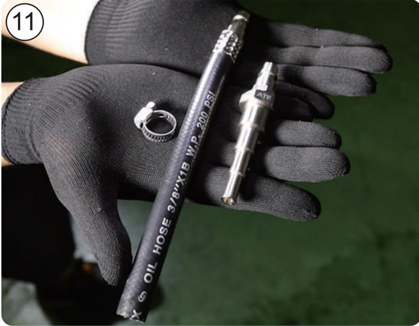
11. Prepare the most suitable adapters (Step adapter, hose, and clamp).
