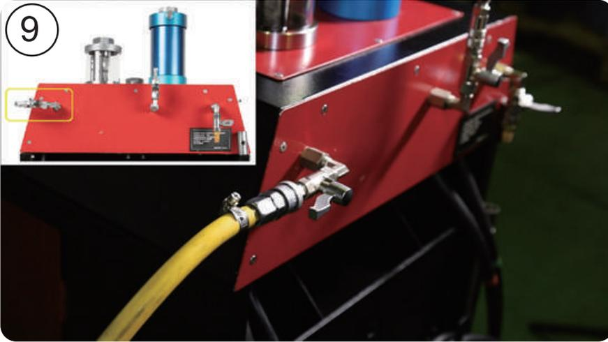
9. Connect the machine to the garage shop air supply.
