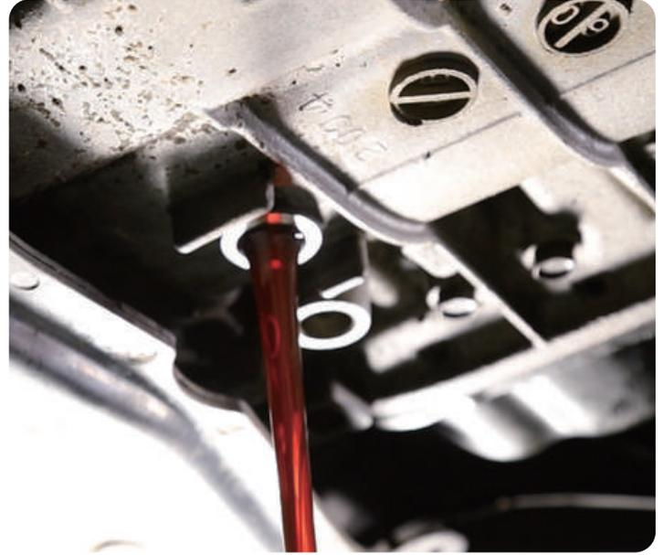
22. Once the ATF is drained completely, lift down the vehicle, and turn on the engine for 1-2 seconds, then turn it off, and do this 3 to 5 times, so you let the ATF pass through the converter.
