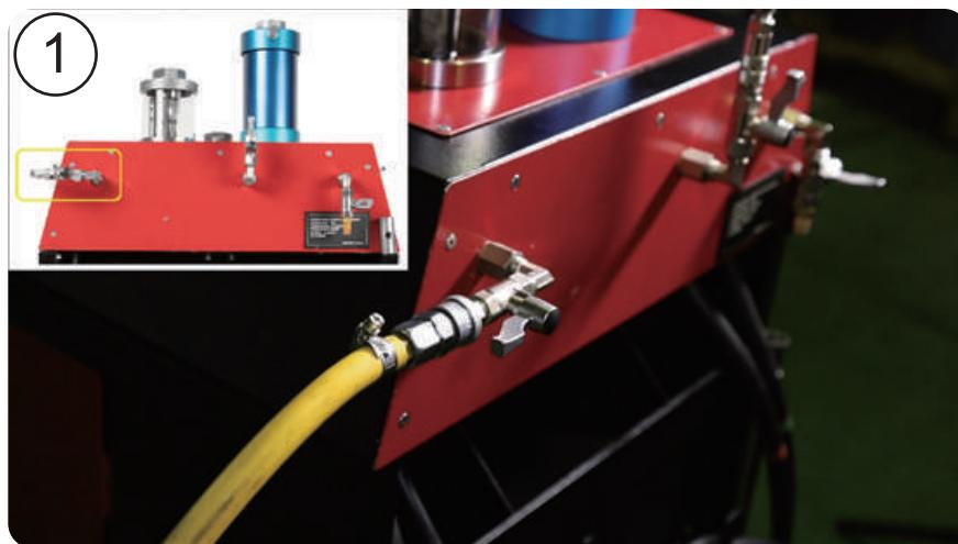
1. Connect the machine to the garage shop air supply.
