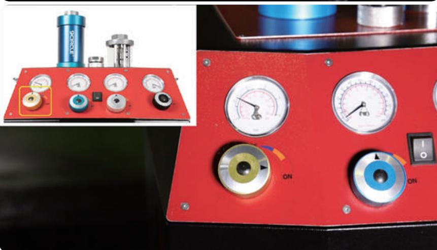
10. Fill ATF (same amount as the amount extracted, which can be seen in the used fluid tank).
