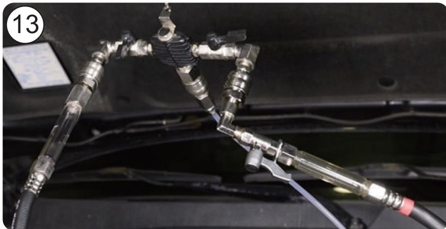
13. Turn off both valves from the black hose side (black hose and T adapter), then turn on the valves on the red hose side.
