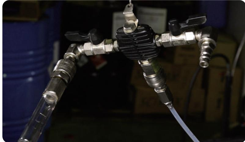
5. To the other side of the T adapter connect the red hose and turn off both valves from that side.
