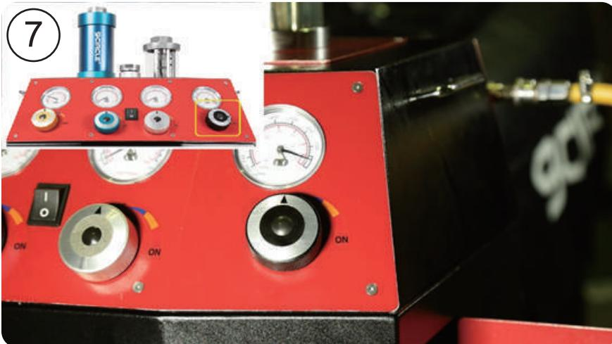
7. Once the machine cannot extract more ATF, turn off the machine's black valve.
