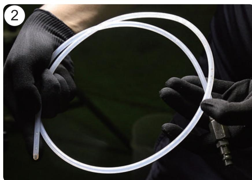
2. Remove the dipstick and install the Teflon tube.
