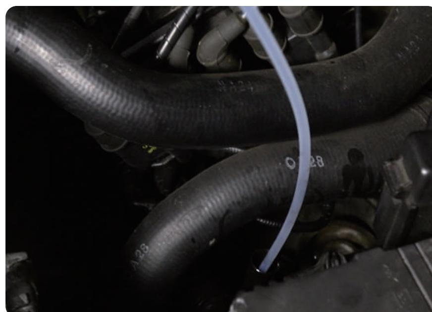
3. Hook the T adapter under the vehicle's hood and connect the Teflon tube plug under the T adapter.
