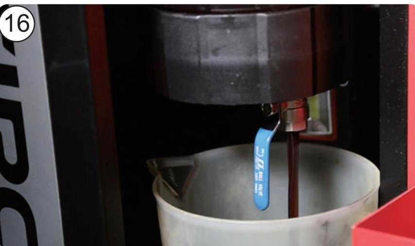
16. Turn on the drain valve from the 5.5L tank, (be sure there is an empty container below the 5.5L tank where the drained ATF can be received).
