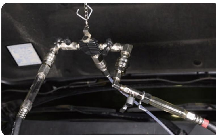
6. Turn on the machine's black valve so can extract ATF.
