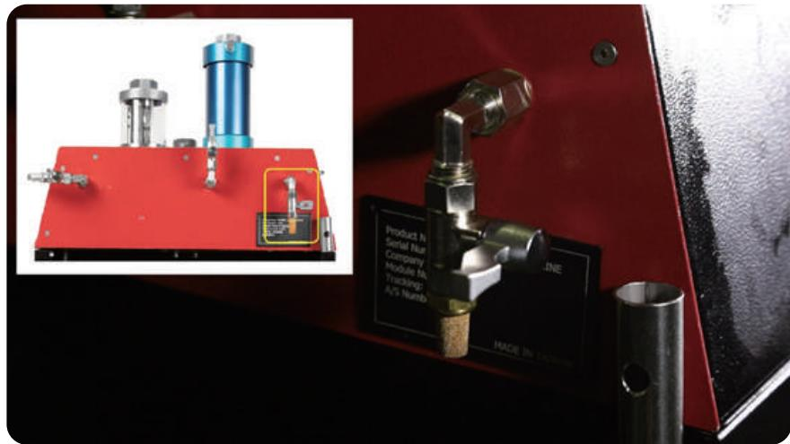
11. After filling the ATF into the 5.5L tank, turn off the golden valve and the machine's rear right valve.
