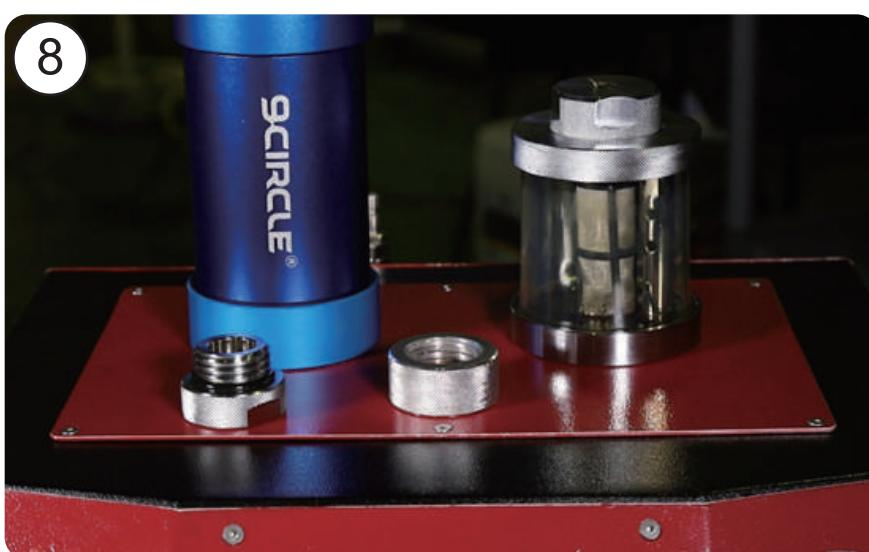
8. Open machine's filling cap and install the funnel.
