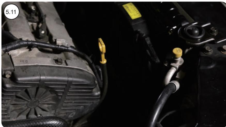
5.11 Install back the engine oil dipstick.
