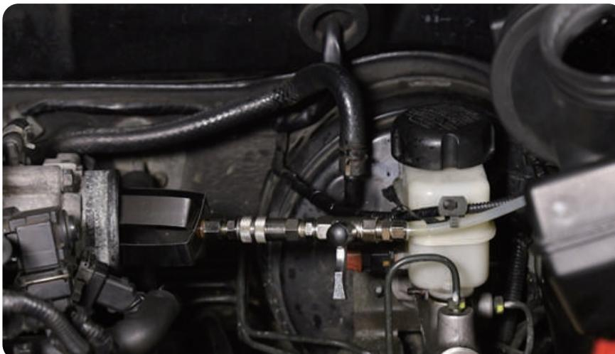
3.4 Connect the other side of the nylon hose (where the clamp is connected), into the machine's rear male coupling. Then turn on the coupling's valve. But keep the clamp's valve closed.
