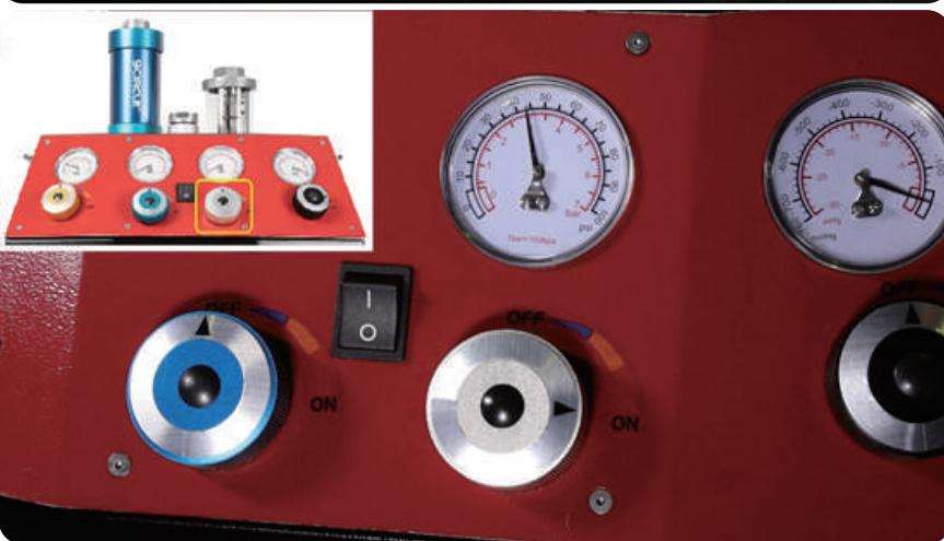
3.9 Oil shower and oil shower 1st time The flush oil will pass through the engine oil line, pouring out the remaining sludge on the engine oil line and oil pan. The air pressure will finish draining all the oil hidden in spaces where the oil is storage and cannot be drain normally.
