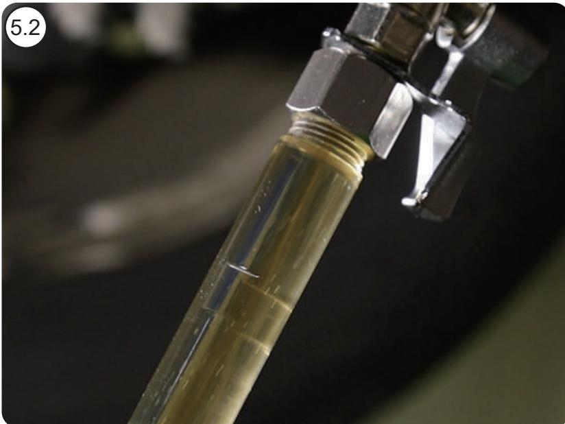
5.2 Disconnect the green hose with its valve open, once is disconnected the machine will suck the remaining oil inside the hose, once there is no oil inside the hose then can close the valve.
