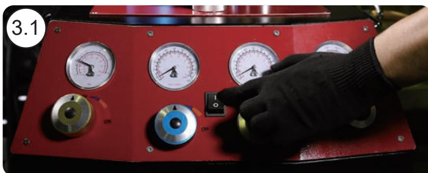
3.1 Turn on the machine's electric motor.
