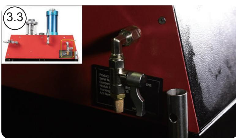
3.3 Turn on the machine's rear right valve, then turn on the front golden valve.
