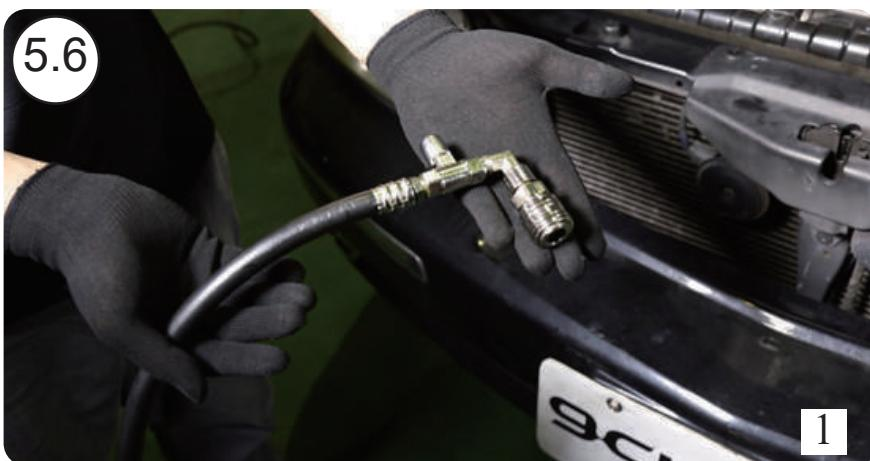
5.6 Connect the black hose (the one without color marks) which is for suction into the nylon tube, push the nylon a little bit to the previous deep, so can suction again, and turn on its valve.
