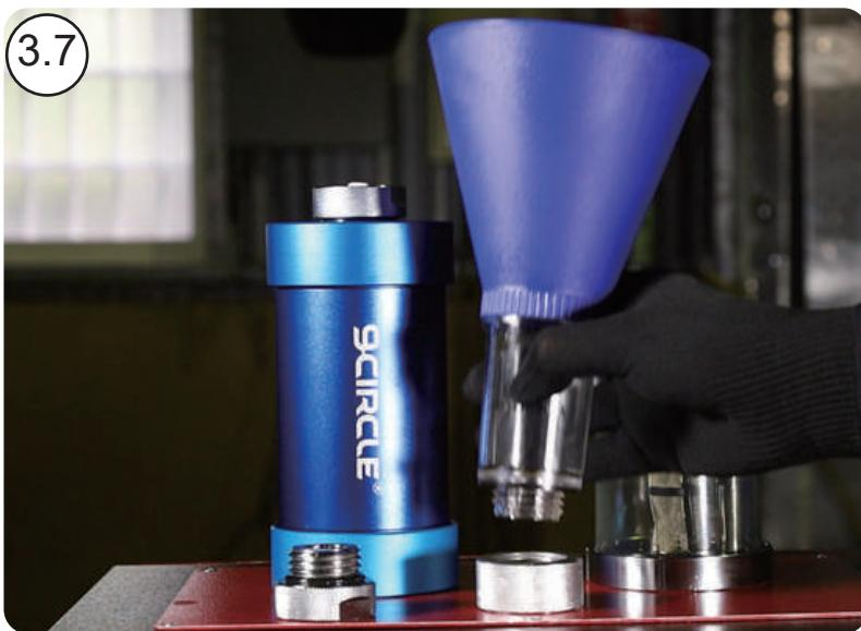
3.7 Disconnect the funnel from the machine, and install back the cap.
