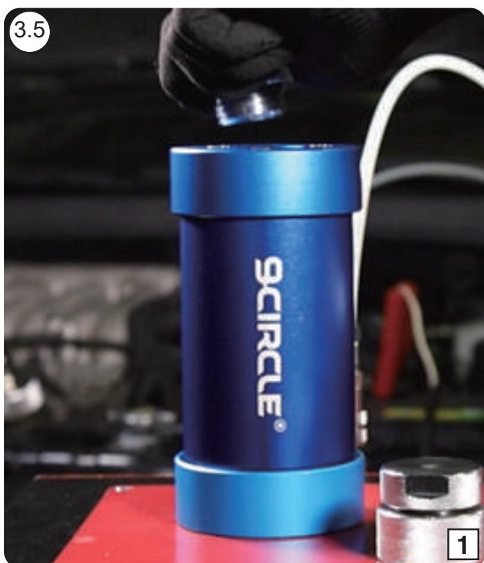
3.5 Open blue cylinder cap, then prepare EXT55 and fill it into the blue cylinder. Then install back the blue's cylinder cap.
