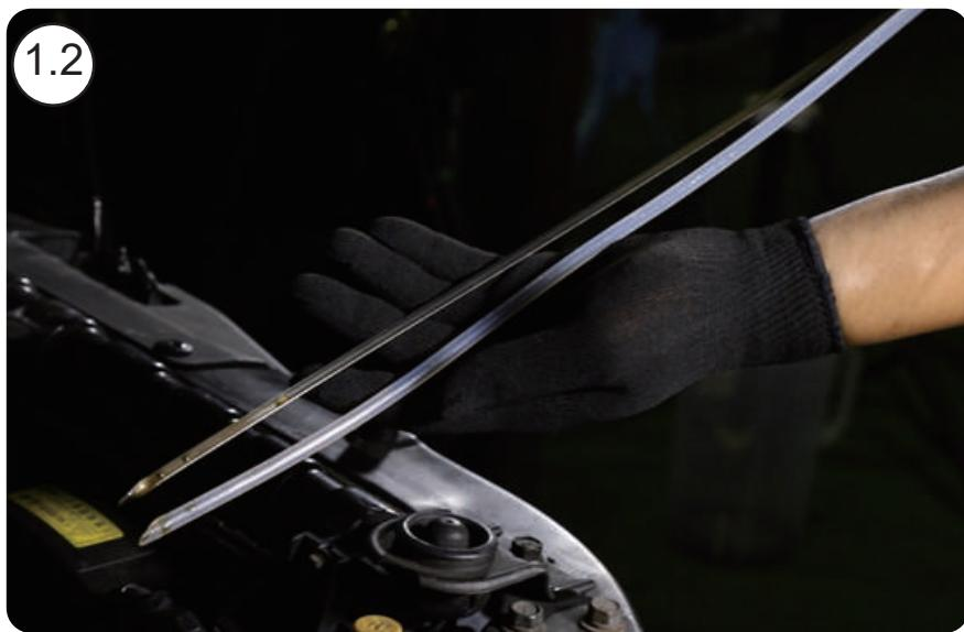
1.2 Chose a suitable nylon tube (to fill and extract oil) and compare its size with the dipstick, then insert the nylon tube into the engine, **please be sure to use the same length as the dipstick.**
