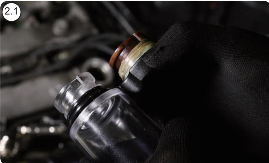
2.1 Open oil filling cap and chose the most suitable engine oil filler neck transparent chamber, then install it onto the engine.
