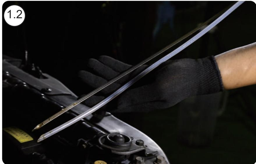
1.2 Choose a suitable nylon tube (to fill and extract oil) and compare its size with the dipstick, then insert the nylon tube into the engine, **please be sure to use the same length as the dipstick.**
