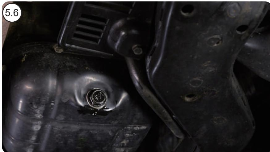
5.6 Install back oil drain plug.
