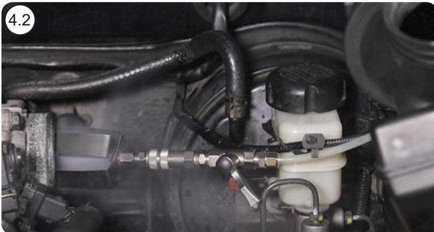
4.2 Turn on spray clamp's valve slowly. EXT55 will be sprayed onto the intake throttle.
