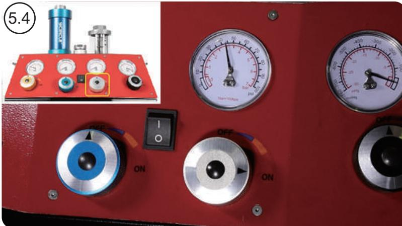
5.4 Turn on the machine's air shower valve (silver valve), which will use air to pour out the remaining oil on the oil pan.
