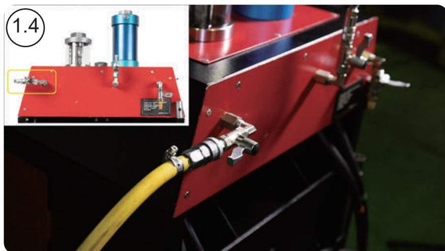
1.4 Connect air supply to the machine. And turn on the valve.
