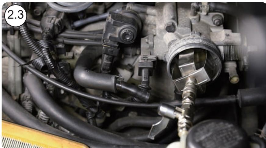
2.3 Connect clamp into intake throttle. Keep the nylon's hose valve closed.
