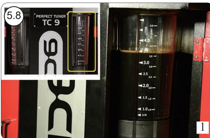
5.8 Once the oil is extracted turn off the suction hose valve, and the machine's black valve and turn on the drain valve from the 5.5L tanks, (be sure there is an empty container below the 5.5L tank where the drained oil can be received).
