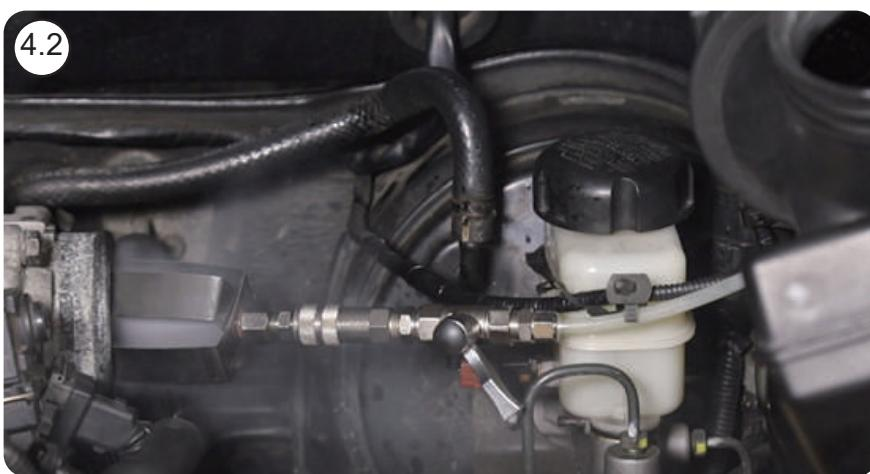
4.2 Turn on spray clamp's valve slowly. EXT55 will be sprayed onto the intake throttle.
