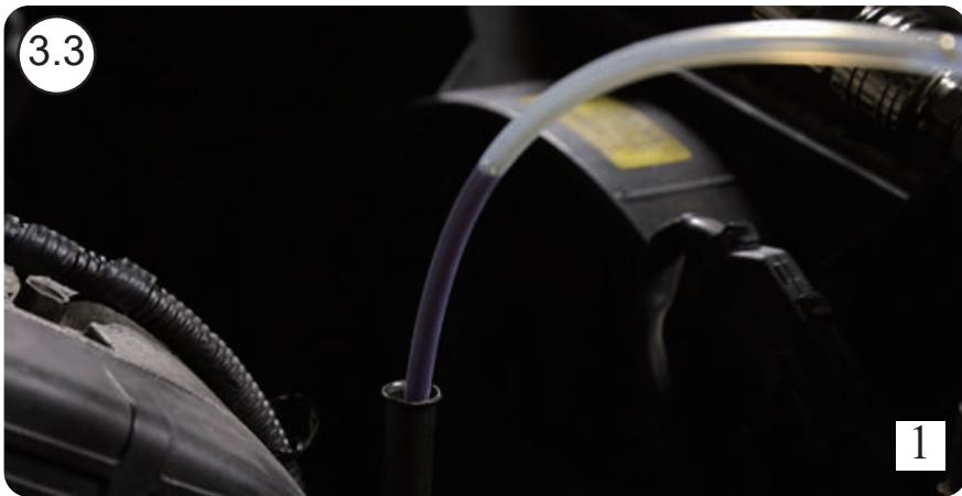
3.3 Used oil is extracted and is sent into to the machine's filter transparent chamber which will show the dirt that is being filtered.
