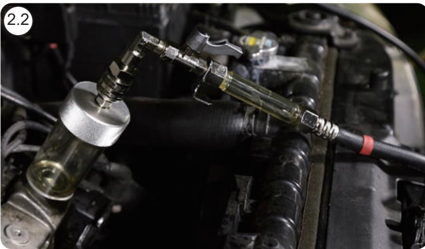
2.2 Connect the filling hose (red) to the engine's oil filler neck transparent chamber. Then turn on the valve.
