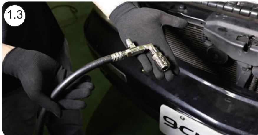
1.3 Connect the flush suction hose (black) with the Teflon tube and turn on the black hose valve.
