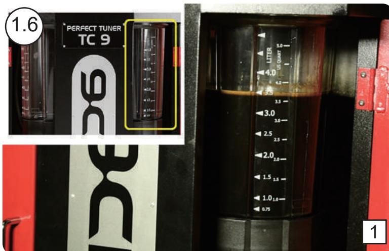
1.6 Once the oil is extracted, turn off the valves, disconnect the black hose, remove the Teflon tube and install back the engine oil dipstick.
