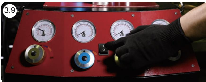
3.9 Turn on machine's electric motor and turn on the machine's blue valve.
