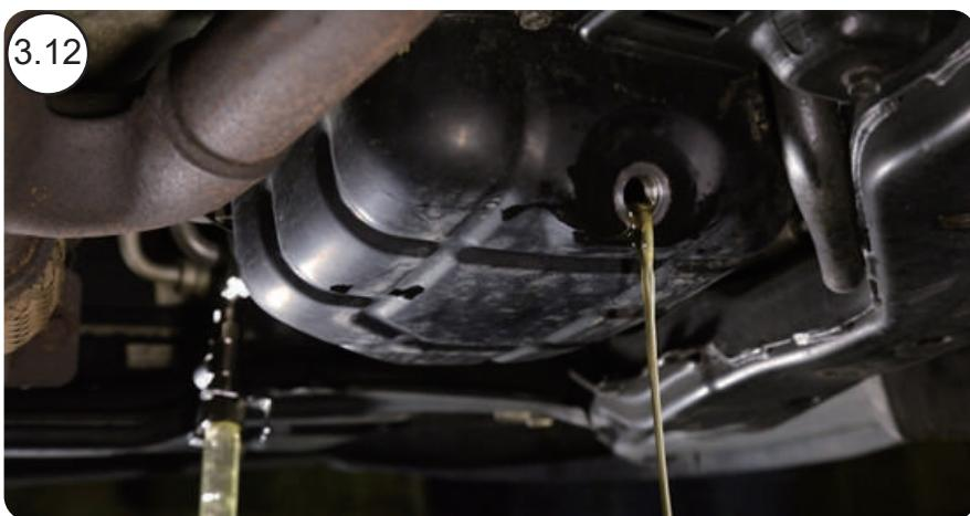
3.12 Repeat the work one last time by filling out the last liter of flush oil. This time the flush oil that goes out from the oil pan should be totally clean.
