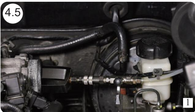
4.5 Turn off the spray's clamp valve and the blue valve from the machine after chemical spraying is finished.
