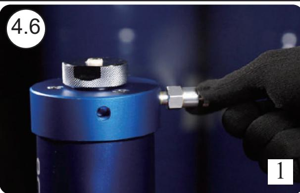
4.6 Turn on release pressure valve from the blue cylinder, observe the gauge and be sure all the pressure has been released. Then turn off the release valve from the blue cylinder.
