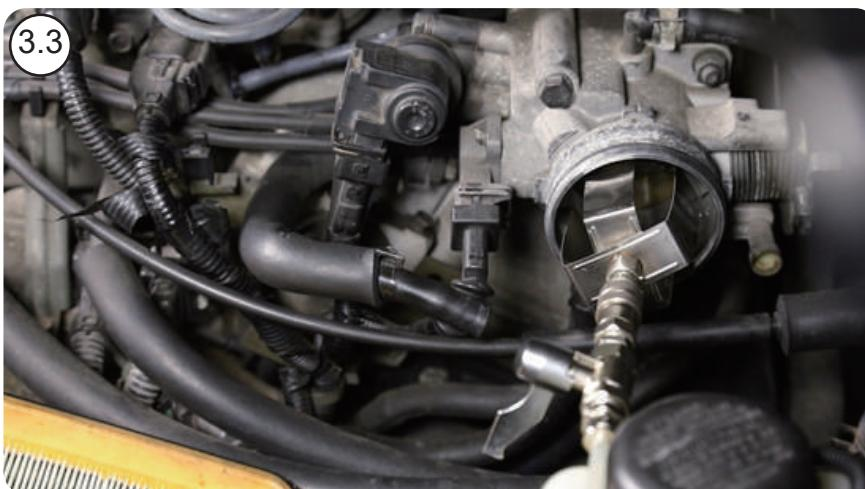
3.3 Connect clamp into intake throttle. Keep the valve closed.
