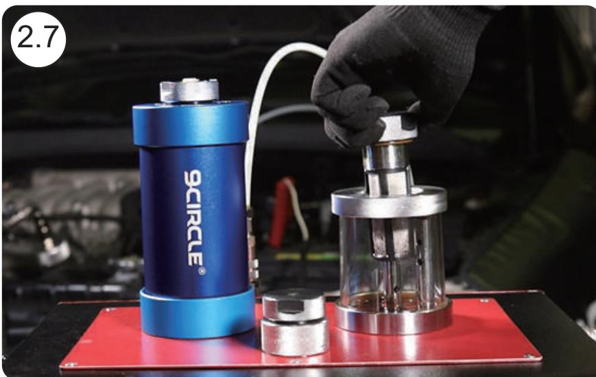
2.7 Open the cap of the machine's filter transparent chamber.
