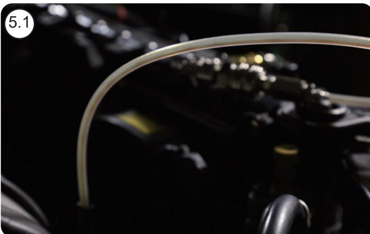
5.1 Turn off the vehicle's engine and then lift the nylon tube a little bit to stop the suction and avoid spill oil when you have to disconnect the hose.
