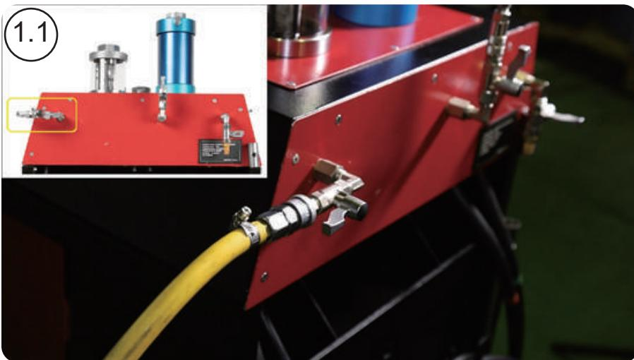
**1.1 Connect air supply to the machine and turn on the valve.**
