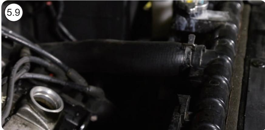
5.9 Remove the engine oil filler neck transparent chamber.
