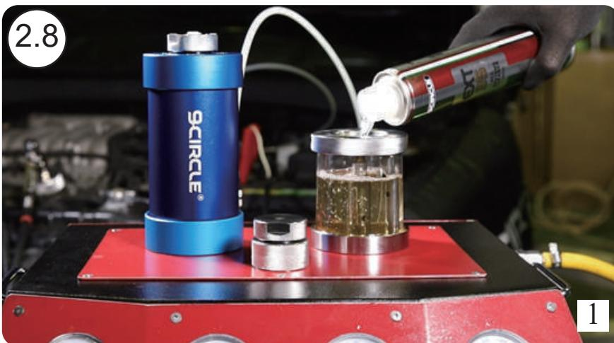
2.8 Prepare EXT35 and fill it into the machine's filter transparent chamber, then put the cap back.
